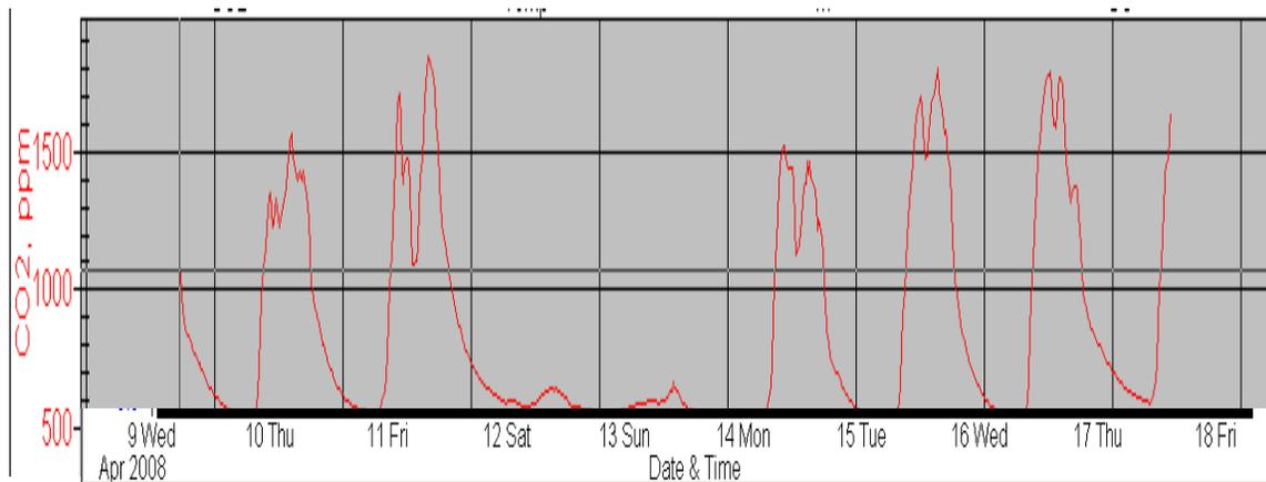
Figure 10. Pilot Building # 2 Carbon Dioxide Concentrations
