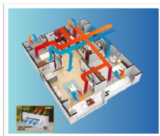
Figure 7: Example of hybrid ventilation system
