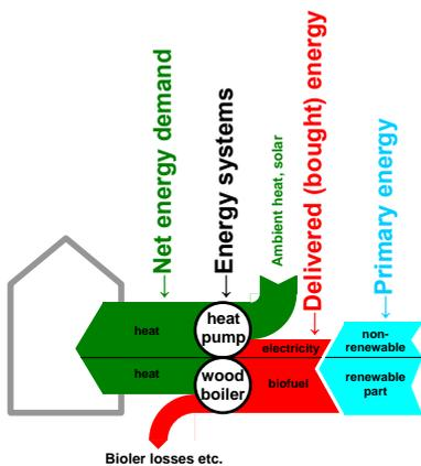
Fig.3: Illustration of net & delivered energy, and primary energy type
