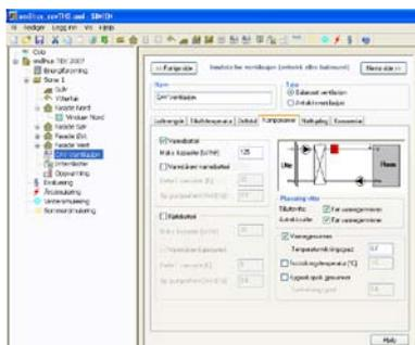
Fig.4: 'SIMIEN' software with dynamic hourly energy calculations according to NS 3031
