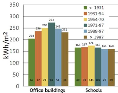
**Fig.19: Present energy consumption of offices & schools by construction year. Buildings from <1931 do not use more energy. Many older buildings in this sample have probably been rehabilitated. The picture for housing is the same. [source: ENOVA]**
