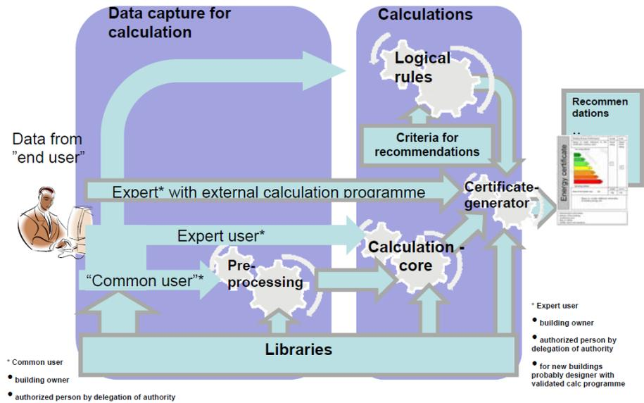
Fig.13: Schematic showing information flow and processing in the Energy Marking System (EMS). [source: Rode & Isachsen, NVE]
