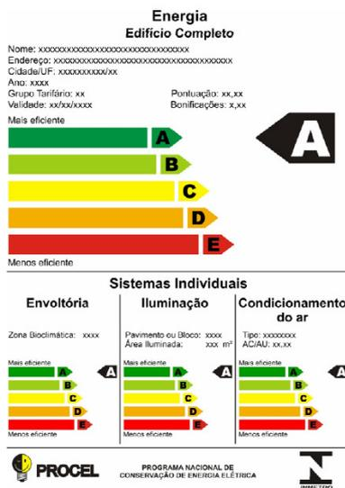
**Figure 1:** Model of the National Label of Energy Efficiency – ENCE. Source: Inmetro (2009a).
