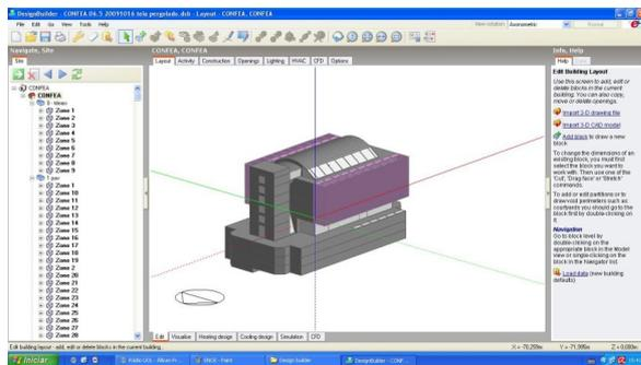
**Fig. 5:** DesignBuilding interface and the building modeling.
